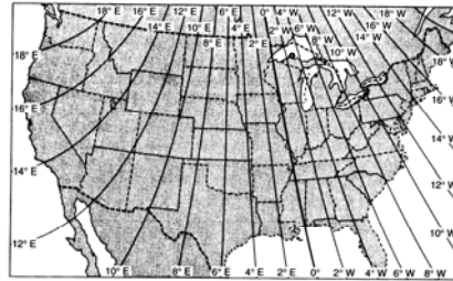
FIGURE 4-3 Magnetic declination chart of the conterminous United States, epoch 2000. (Figure produced by L. R. Newitt, Geological Survey of Canada, Natural Resources Canada, using data from Geomagnetic Reference Field 2000.)
